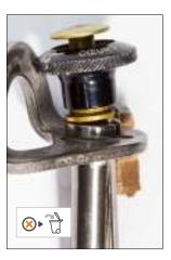
• Marked and deformed plunger
